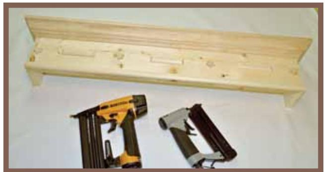
Fill any holes and seams with wood putty and let dry. Sand with sandpaper and steel wool. Remove any sawdust with a slightly damp rag.
