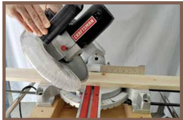
Use the outside measurements of the dust cap for the inside miter measurement for the face boards. For this example, I'm using a 1x6 board for the face. Cut the face board first. To cut the returns, lay the face board facedown, place the dust cap on top of it in the proper position, then hold the mitered return section next to the dust cap return and mark where the return is to be cut.
