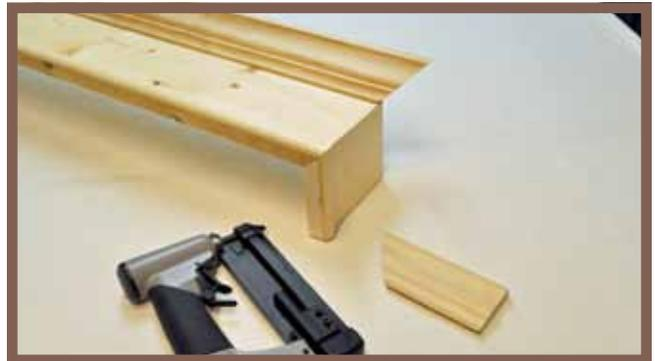
Add any embellishments in the desired locations using the pin nailer. This photo also shows a brad nailer on the left and a pin nailer on the right.
