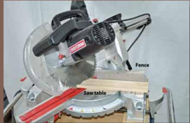
B. Outside corner – right side. Lay the molding face side up flat on the saw table and the top of the molding against the fence. Set the bevel setting at 33.9 degrees. Set the miter table at right 31.6 degrees, the molding to the right of the blade is the finished piece. ✨
